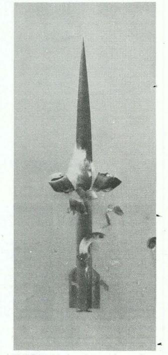
HIGH ALTITUDE research projectile was photographed by an image motion camera as it left muzzle. Photo shows sabot separating from the unit. Velocity of projectile at this point was 4946 ft. per second.
